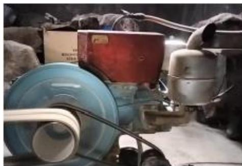
Gambar 2. Mesin diesel Dongfeng type R175
